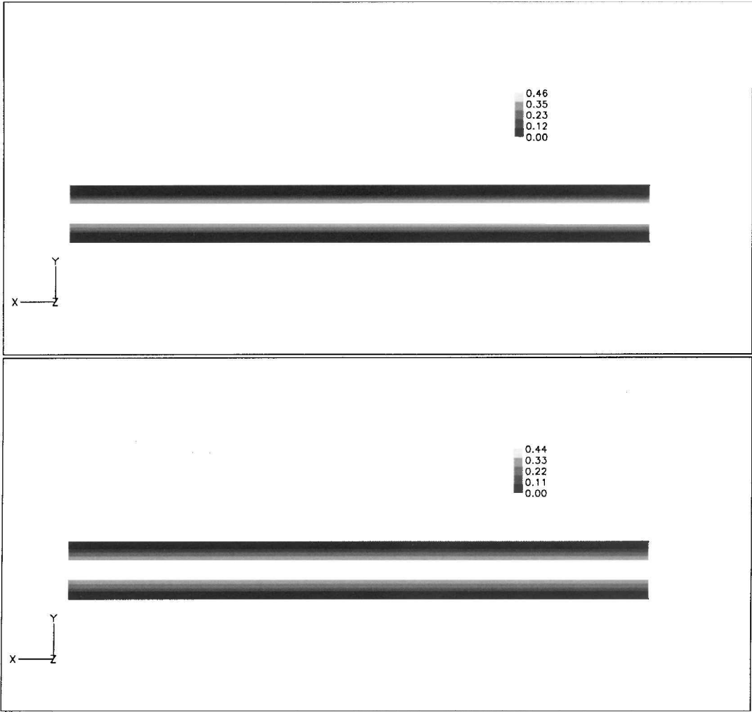
Fig. 4 Collection efficiency at the surface of a two-dimensional cylinder for one MVD = 16 μm solution (top) and a Langmuir-D distribution with the same MVD (bottom).
